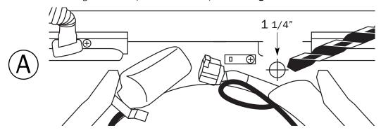
3. Route the included cables through the hole and install the supplied rubber grommet on the cables and into the  $1\,1/4$ " hole.
