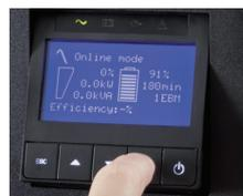
9SX LCD tilts 45° for ease-of-viewing
